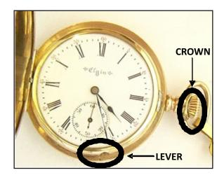
To wind your watch, grasp the grooved crown that juts out from the frame of the watch between your fingers and gently turn it clockwise. You should hear a repeating 'click' sound as it turns. Continue to wind the watch until you begin to feel some resistance. You can over wind and damage the watch if you try to force the crown to turn, so take it slow for the first few days you have your watch until you get a feel for how much you can wind it.
